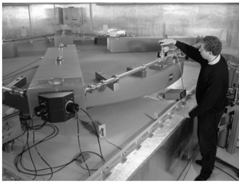
Figure 6. Picture of the G ring-laser located in Wettzell on its zerodur support; the apparatus is shown without the temperature and pressure controlled casing that covers it when in operation.
