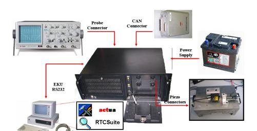
Figure 10.3. PZO Driver rack and its interfaces
