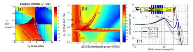
Fig.1.(a) Frequency separation map and (b) intensity modulation responses map, calculated for  $x_A = 0$  and values of the normalized parameter  $x_P$  ranging from -0.5 and 0.5, for an as-cleaved CCIG with  $L_A/L_G/L_P = 200/600/10 \ \mu\text{m}$ . (c) Cuts of the map reporting the IM responses for several values of  $x_P$ . In the inset, a scheme of CCIG is reported.
