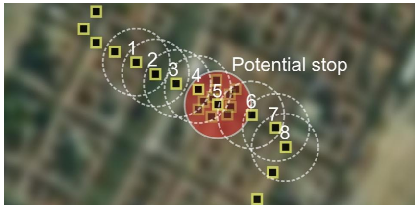
Figure 37 – Example of trip/stage detection according to point spatial distribution
