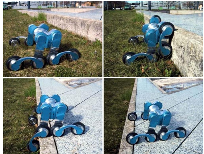
Figure 7. The leg-wheel hybrid Octopus robot (Lauria et al., 2002).
