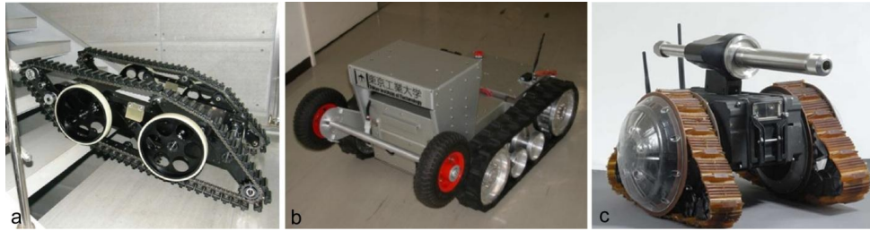
Figure 10. Wheel-track hybrid robots: with variable-shape tracks (a, Kim et al., 2010); Helios VI (b, Hirose et al., 2001); with Galileo wheel (c, http://www.galileomobility.com ).
