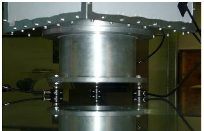
Figure 9. The interface adapter, that supports the nanosatellite engineering model, and the air pad system, attached to the bottom of the interface adapter.
