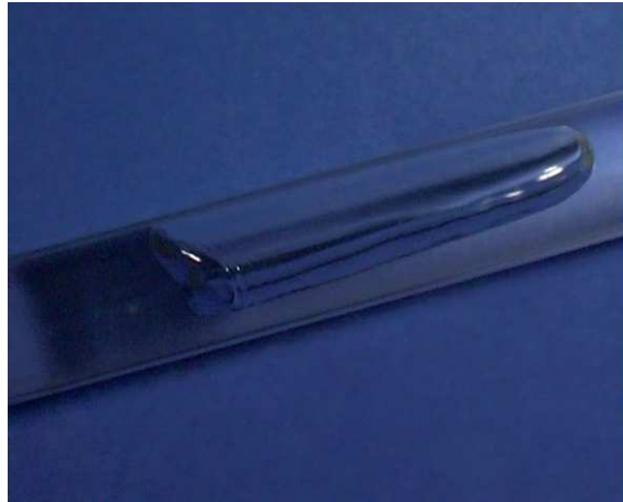
Figura 116: W_{\text{acqua}} = 200 \text{ l/h} e W_{\text{aria}} = 50 \text{ l/h} \Delta z \sim 2 \text{ m} ; elica D = 1 \text{ m} . Circuito A.
