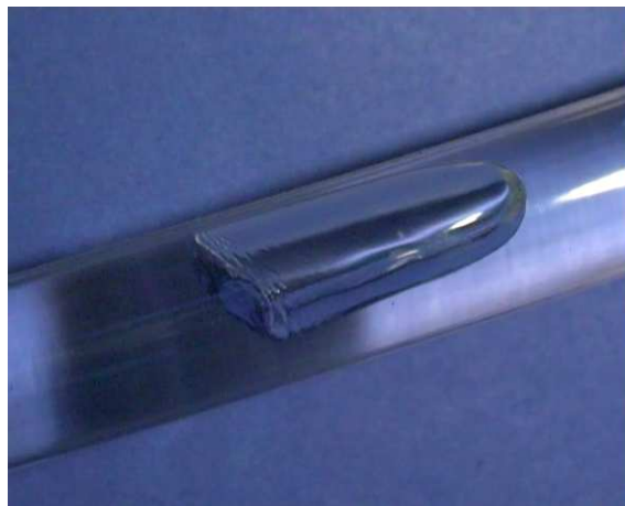
Figura 115: W_{\text{acqua}} = 200 l/h e W_{\text{aria}} = 50 l/h \Delta z \sim 1,25 m; elica D = 1 m. Circuito A.
