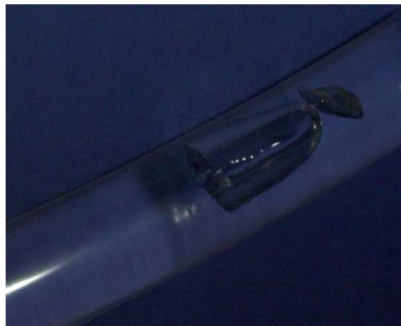
Figura 114: W_{\text{acqua}} = 200 l/h e W_{\text{aria}} = 50 l/h \Delta z \sim 0,45 m ; elica D = 1 m. Circuito A.
