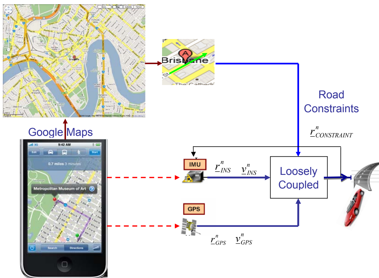
Figure 7. A closed-loop Loosely Coupled GPS/INS integration scheme with constraint.
