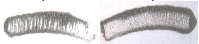
Fig. 5 – Magnetized samples: left parallel, right radial
