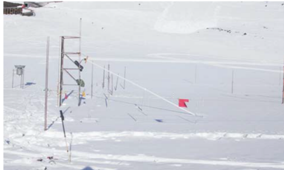
Figure 2.5: Final configuration of the TDR measurement, with the cable deployed along the slope
