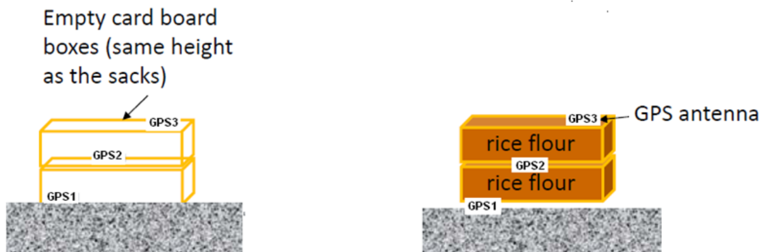
Figure 4.36: Lateral view of the used measurement configurations. On the right the experiment with rice sacks and on the left, the same configuration, but with empty boxes
