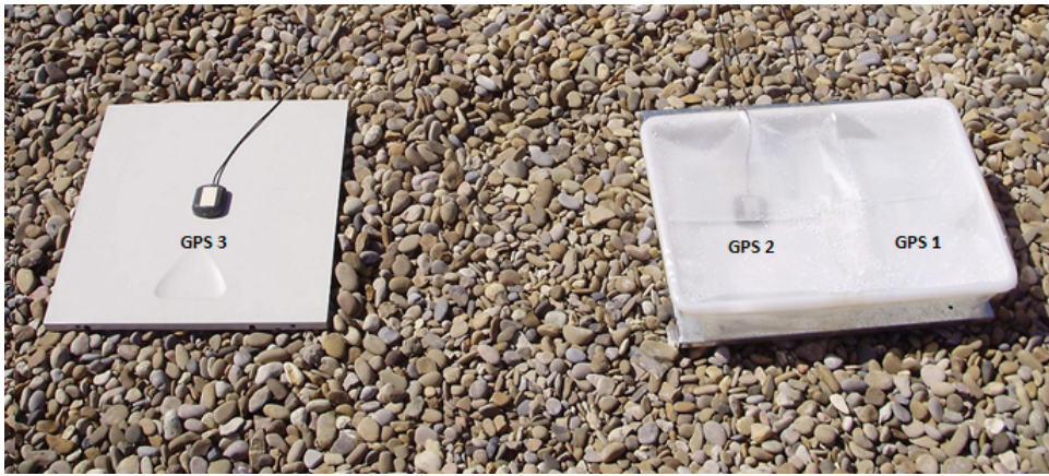
Figure 4.13: Detail of the GPS receivers configuration. On the right GPS1 and GPS2 inside and under a box containing water and, on the left, GPS3 in a standard free space configuration
