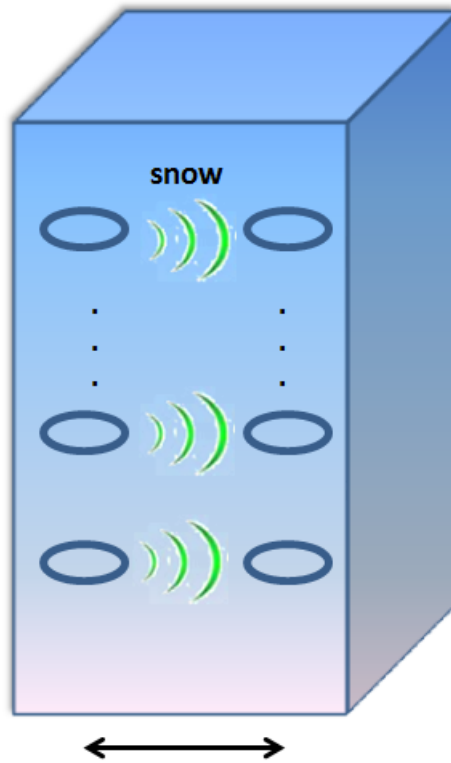
Figure 3.2: Schematic view of the sensors buried into the snow - magnetic radiators
