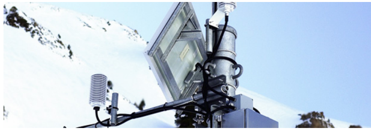
Figure 2.3: View of the cosmic ray gauge for the snow water equivalent estimation
