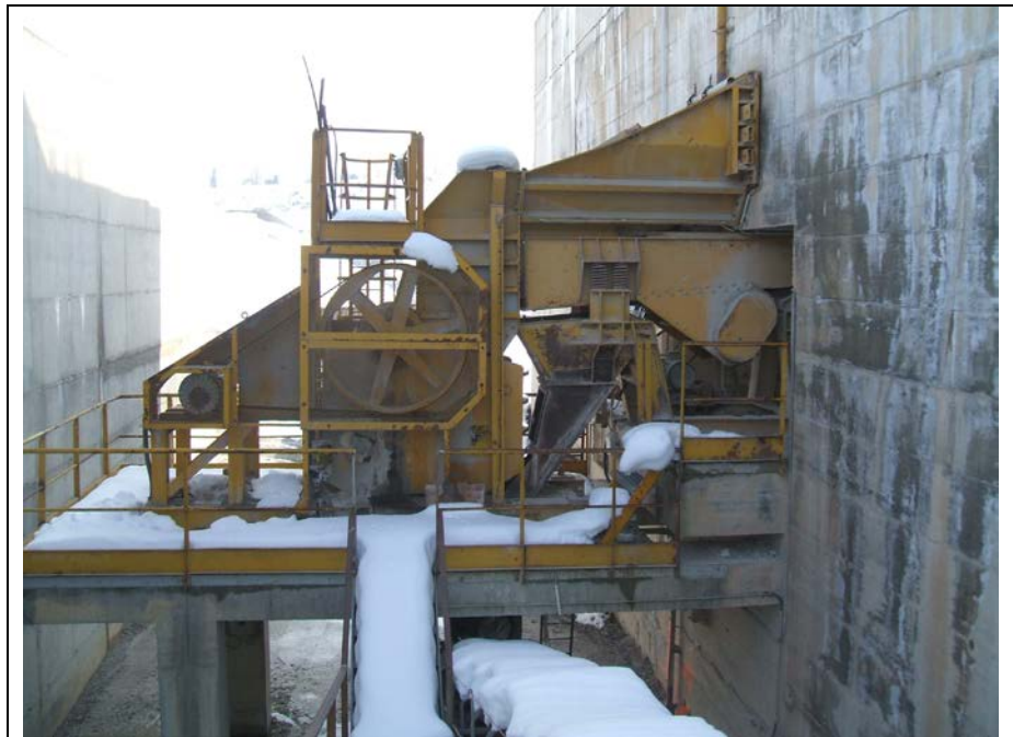
Figure 7.15: Side view of the primary jaw crusher
