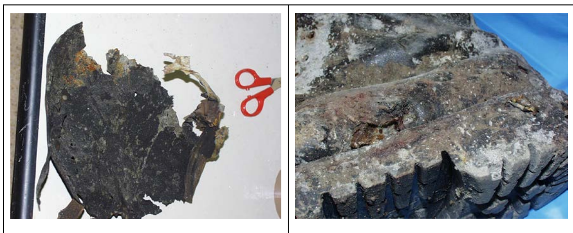
Figures 5.6 and 5.7: Parts of the metal tank ripped by the explosion which were found stuck in the boot of the victim
