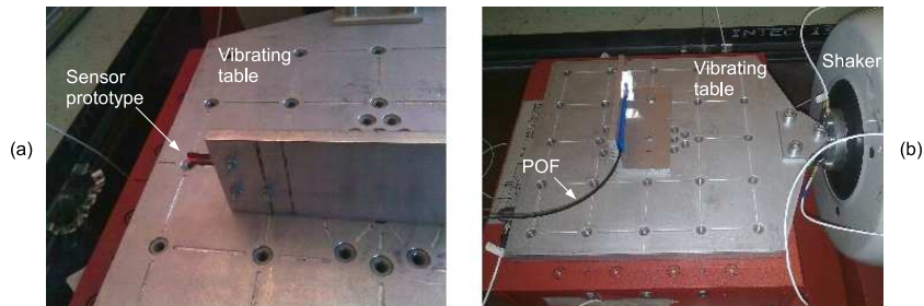
Figure 7.11. Setup employed to test the prototype without grooves in reflection mode: lateral (a) and front view (b).
