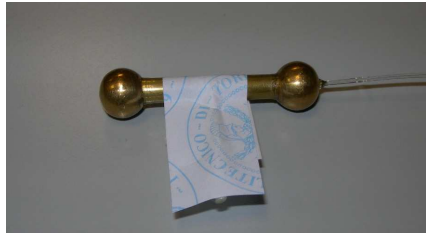
Figure 4.7. POF sensor ready to be installed in the Chapel.
