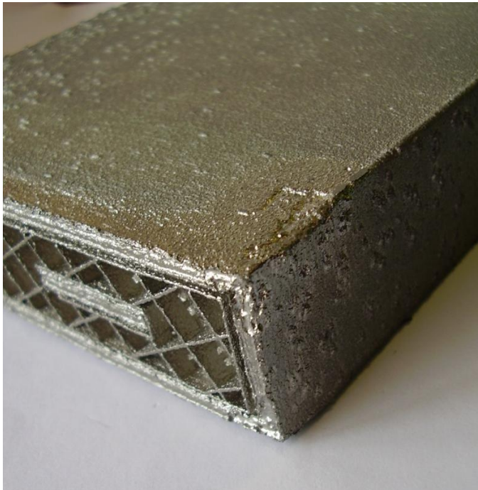
Figure 1: EBM sintered workpiece, as supplied
