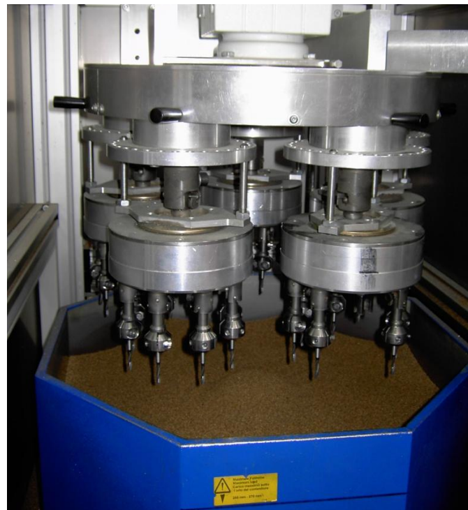
Figure 5: OTEC DF 70 drag finishing machine.
