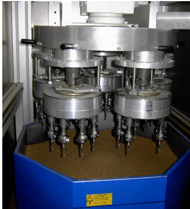
Figure 5: OTEC DF 70 drag finishing machine
