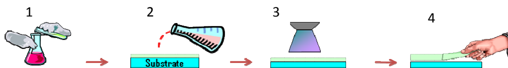
Figure III. 3. Scheme of the preparation of the membrane
