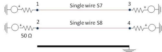
Figure 3: Test configuration of a 4-port measurement on single wires S7 and S8
