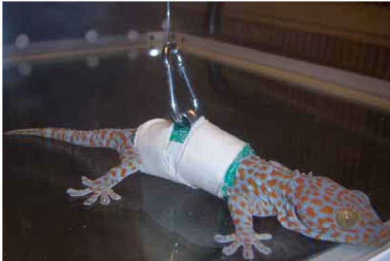
Fig. 3.4 Our tested Tokay gecko: adherent elastic cloth bandaging and metallic hook of connection with the outside measurement platform.
