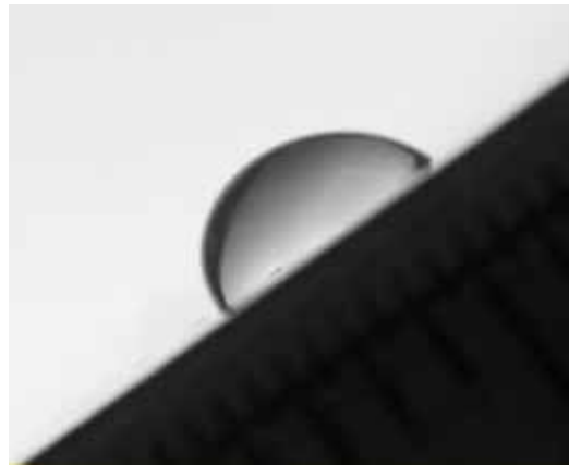
Fig. 6.9 Sample 4B i at 36°, the sliding was observed at 48°.
