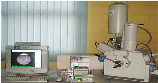
**Figure 2.** Scanning electron microscope (SEM)
