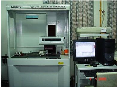
**Figure 1.** Formtracer CS-5000.
