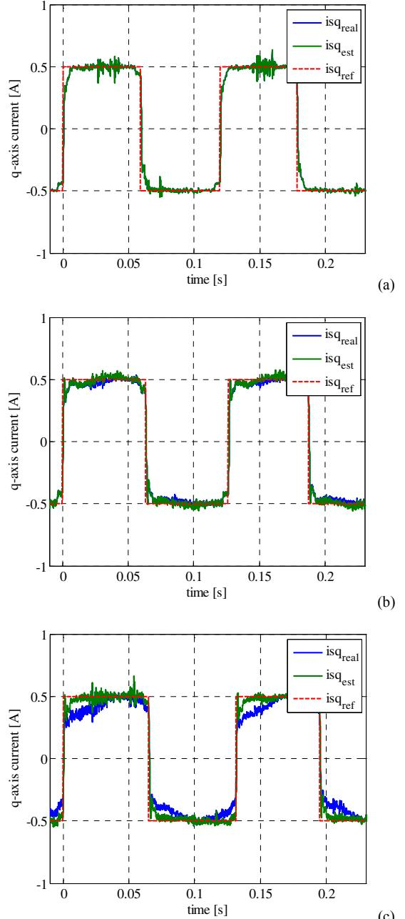
Fig. 9 –  $i_{sq}$  current responses using (a) sensorless control, (b) sensorless control based on pulsating voltage injection with the proposed compensation LUT, and (c) sensorless control without compensation of the phase of the filters.
