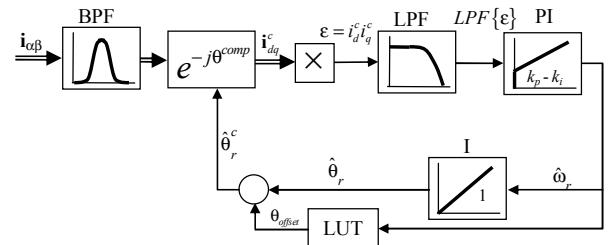
Fig. 2- Tracking observer used with pulsating voltage injection scheme and feed-forward compensation of the BPF delays via a look-up table.
