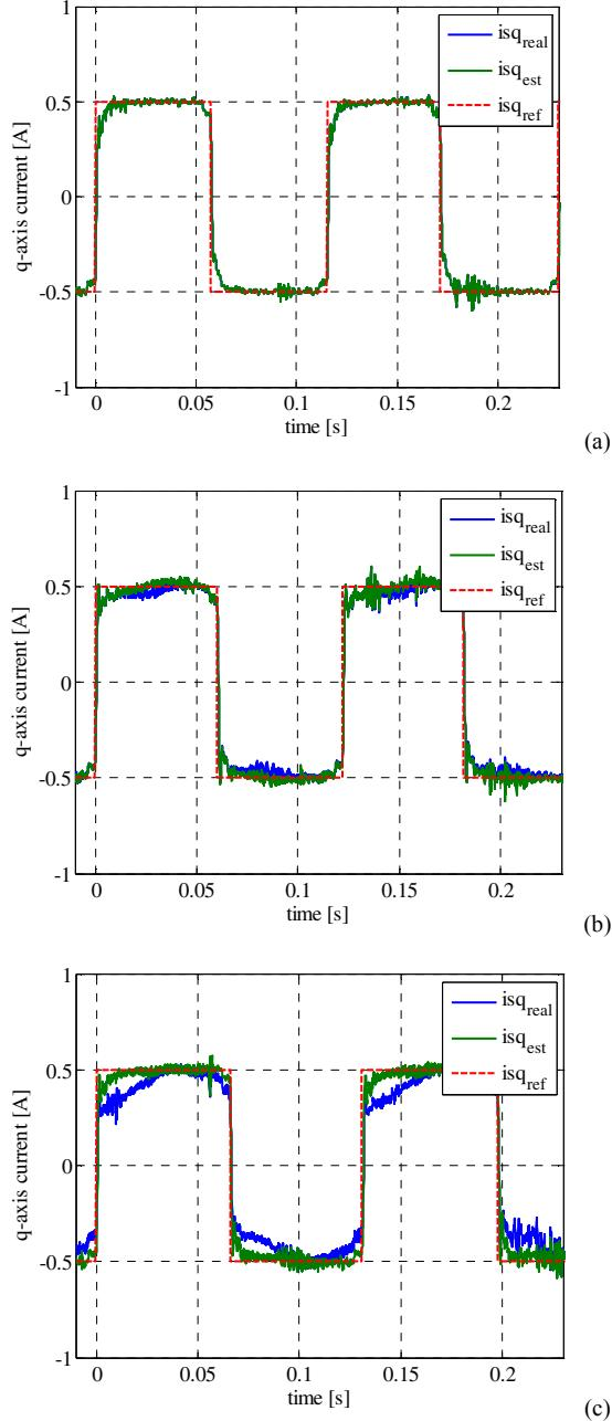
Fig. 8 –  $i_{sq}$  current responses using (a) sensorless control, (b) sensorless control based on rotating voltage injection with the proposed compensation-LUT, and (c) sensorless control without compensation of the phase of the filters.
