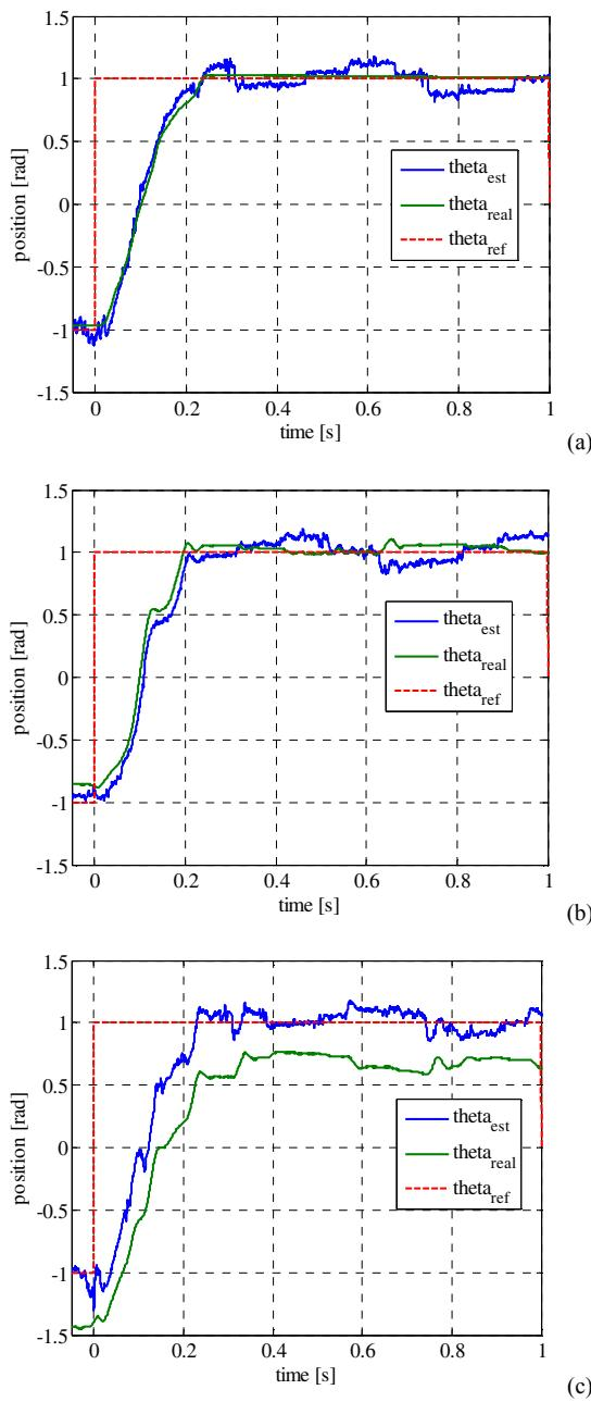
Fig. 10 – Position responses using sensored control (a), proposed sensorless control (b), sensorless control without compensation of the phase of the filters (c).
