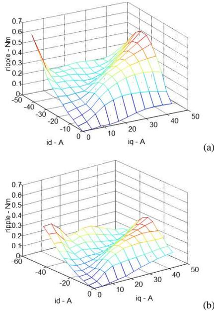
Fig. 4. Torque ripple maps over the  $i_d - i_q$  plane for (a) the GS-solution and (b) the LS-solution.
