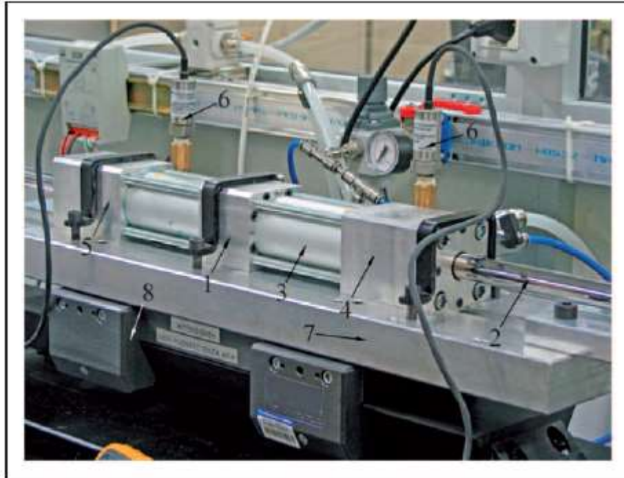
Figure 7: Rod seal friction measurement fixture
