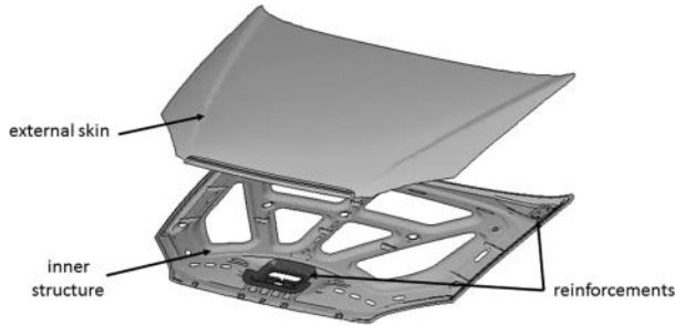
Figure 1. Structure of the reference steel bonnet.
