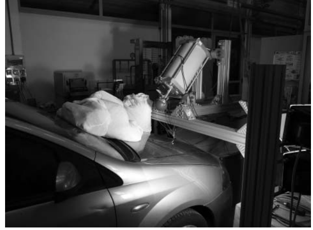
Figure 6. Experimental equipment for the pedestrian head impact tests.
