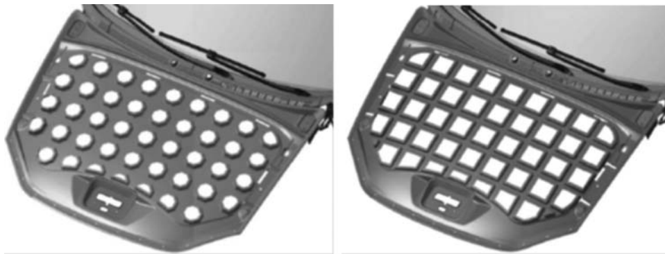
Figure 2. Different designs considered for the thermoplastic inner structure.
