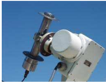
Figure 32 Normal Incidence Pyrheliometer (NIP) (Pyrheliometer s.d.)
