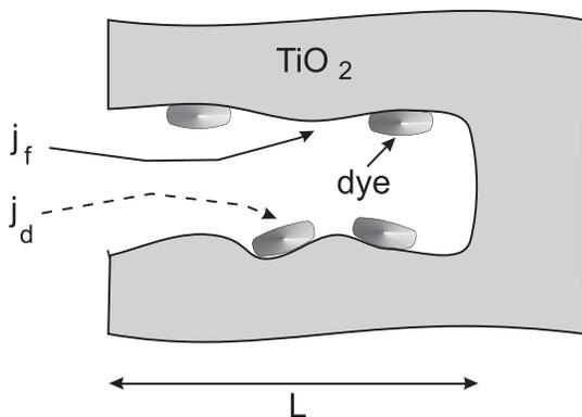
FIG. 1. Schematic representation of a pore of the nanostructured TiO<sub>2</sub> electrode covered with dye.
