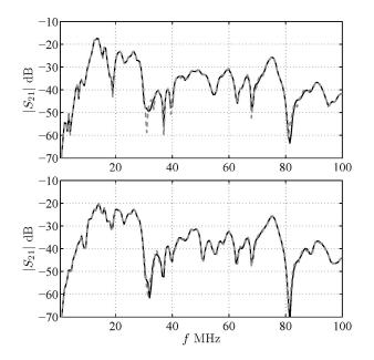
Fig. 6. Magnitude of the  $S_{21}$  scattering parameters of a selection of two alternative measurements. Solid black: measurements; dashed gray: model responses.
