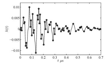
Fig. 3. Automatically selected peaks of the impulse response of Fig. 2 (see the circles superimposed to the impulse response). The abscissas of the selected peaks are the delay parameters of model (1).
