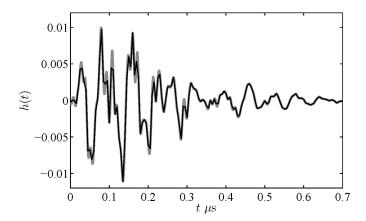
Fig. 2. Impulse response obtained via the inverse FFT of the measured  $S_{21}$  parameter. Black curve: direct application of the *ifft* Matlab function; Gray curve: response with increased time-resolution obtained by zero-padding the original frequency domain response up to 1 GHz.
