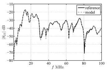
Fig. 5. Magnitude of the  $S_{21}$  reference scattering parameter. Solid black: measurement; dashed gray: model response.
