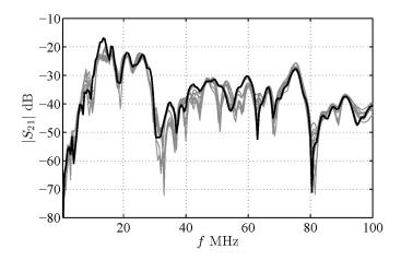
Fig. 1. Magnitude of the  $S_{21}$  scattering parameter of a channel between the outside view mirror controller and the rear left light. The frequency range is [500 kHz,100 MHz]. The thirteen curves in the plot correspond to different possible operating states of the car (e.g., engine turned on or off,...). The black thick line is the first measured curve in the set that has been selected for the application of the proposed technique.
