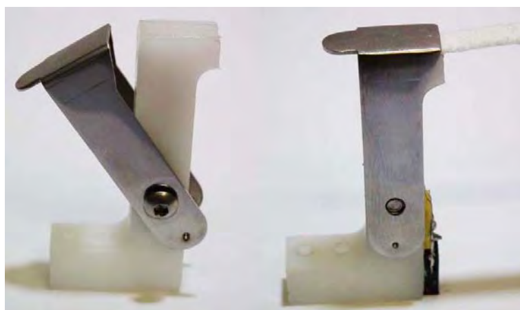
Fig. 109. CPDCD prototype grip system in open (left) and closed (right) position.
