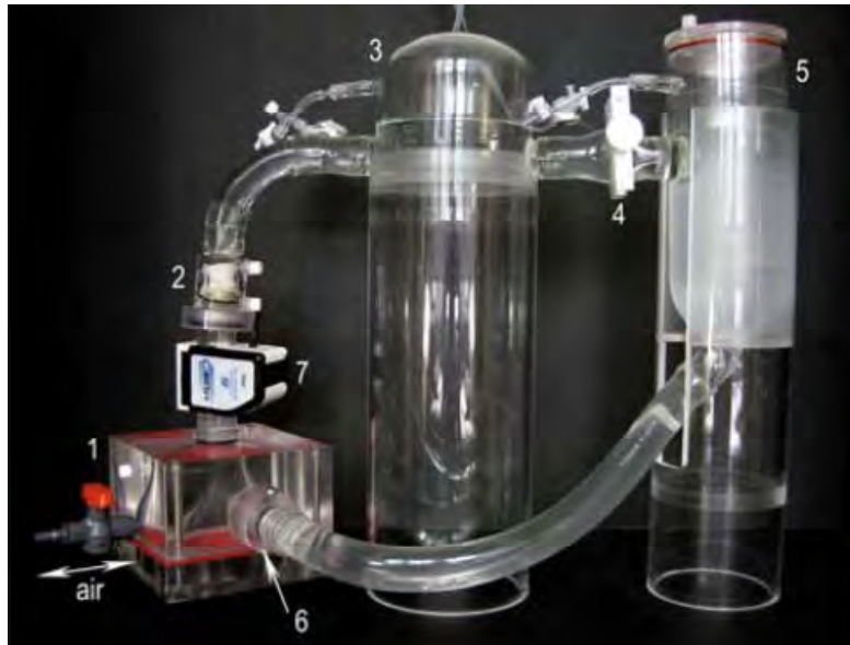
Fig. 66: Bioreactor elements: ventricular pump (1), valve holder (2), compliance chamber (3), variable resistance (4), reservoir (5), bi-leaflet unidirectional valve (6), and flow sensor (7). The compliance chamber (component 3) is located between the valve holder and the variable resistance (component 4) to provide elasticity to an otherwise mostly incompressible system. The role of this location is to simulate aortic and arterial compliance. A custom designed bi-leaflet checkvalve (component 6), represented in detail opens to allow fluid to enter the pump when the membrane moves downward, and closes during systole as the membrane moves upward and flow is produced in the circuit (205).
