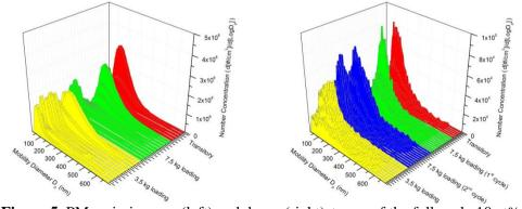
**Figure 5.** PM emissions up-(left) and down-(right)stream of the full-scale 10wt% catalyzed monolith, for 7.5 and 3.5 kg wood-loadings. Dilution factor ~ 60.
