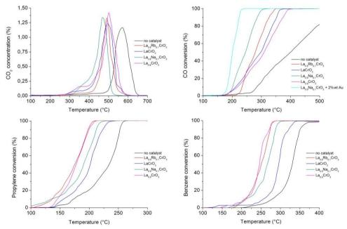
**Figure 3.** From left to right, and from top to bottom: soot, CO, propylene and benzene oxidation tests (see the text for detailed experimental conditions) with powder catalysts.
