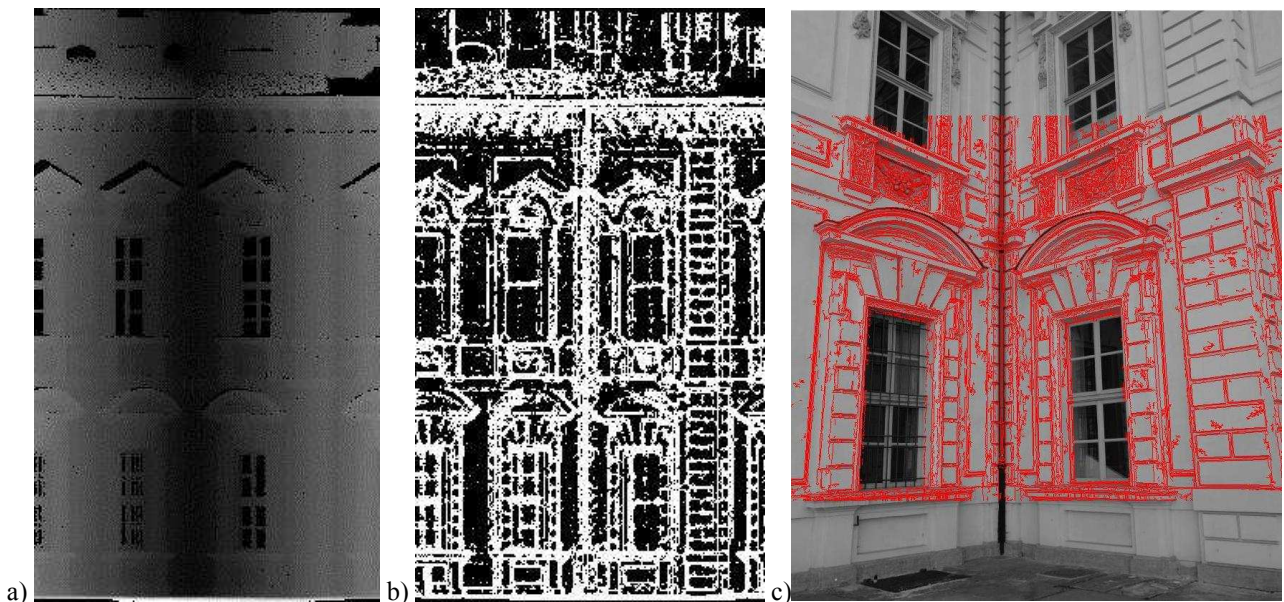
Figure 11. Regularized DSM (a), corresponding region of interest (b) and extracted edges (c).
