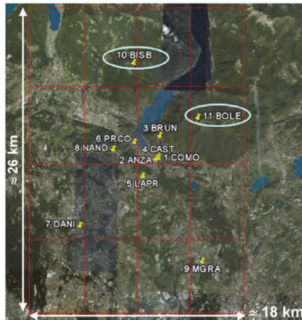
Fig. 3. Geographic distribution of the MisT network. The two “mountainous” GPS receivers are highlighted. The final volume discretization is also superimposed.
