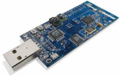
Figure 3: Tmote Sky wireless sensor module
