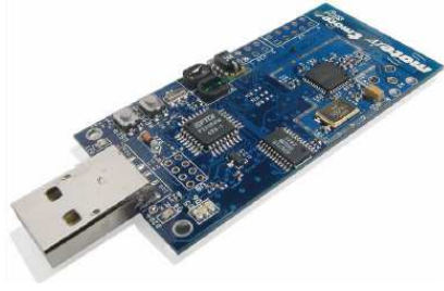
Figure 3: Tmote Sky wireless sensor module
