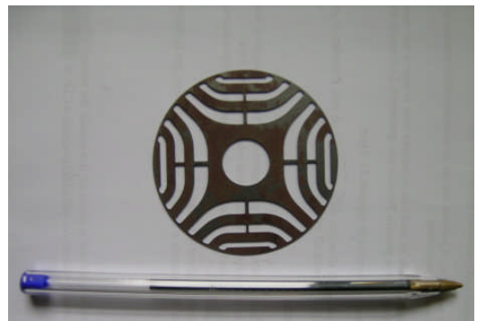
Figure 7. Rotor lamination of Motor 1. The PM bonded (ferrite) material is injected in the hollow flux barriers
