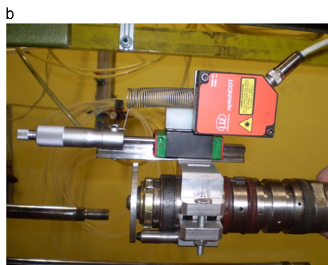
Fig. 2. Wear measuring device, equipped with a laser displacement sensor: (a) scheme; (b) manufactured equipment.
