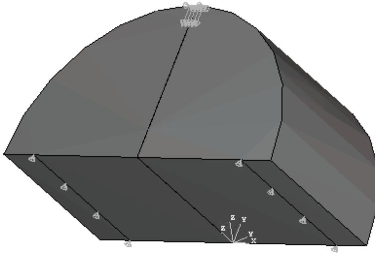
Figure 7: Boundary conditions applied to the solid model
