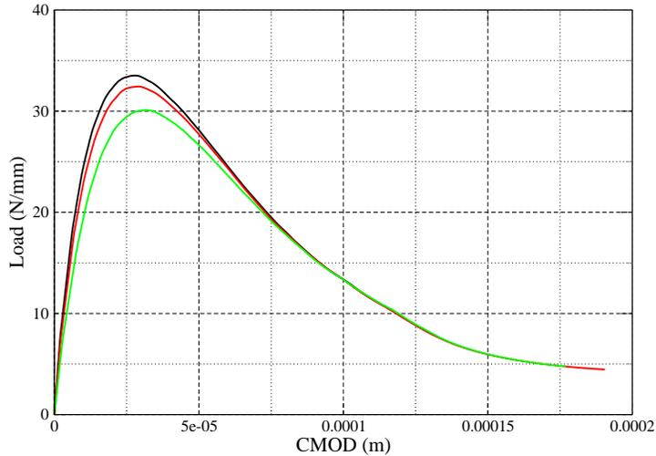
Figure 9: Load per unit specimen thickness vs Crack Mouth Opening Displacement plot per unit specimen thickness; upper curve  $a_0=5.4$  mm, middle curve  $a_0=6.0$  mm, lower curve  $a_0=7.3$  mm
