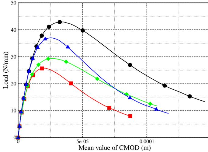
Figure 10: Sensitivity of load vs CMOD diagram on  $f_t$  and  $w_m$  ( $a_0=6$  mm); (a) a circle indicates both parameters increased of 25%; (b) a triangle indicates  $f_t$  increased and  $w_m$  decreased; (c) a rhombus indicates  $f_t$  decreased and  $w_m$  increased; (d) a square indicates both parameters decreased of 25%;
