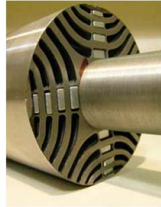
Fig. 4 – Permanent-Magnet Assisted Synchronous Reluctance (PMASR) rotor during motor assembling.
