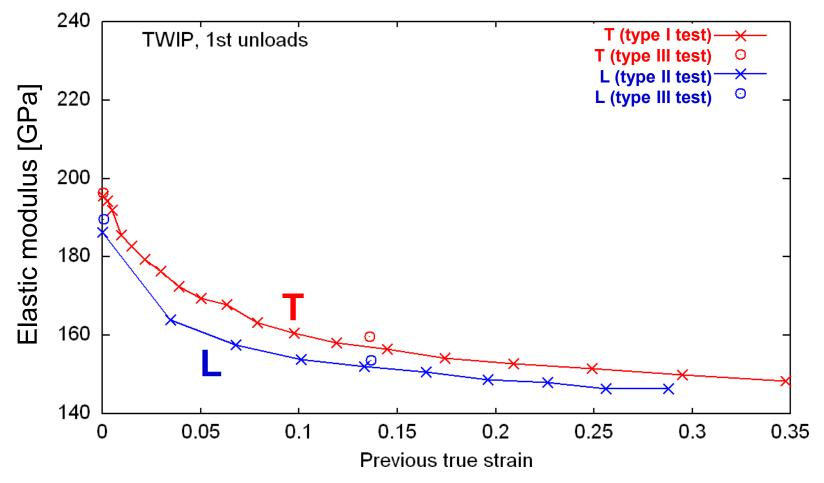
A small difference due to the specimen orientation can be detected in most examined materials
