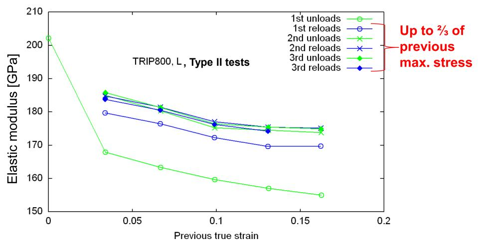
Differences are slightly broader than in type I tests, probably due to the lower reloading max. stress.
