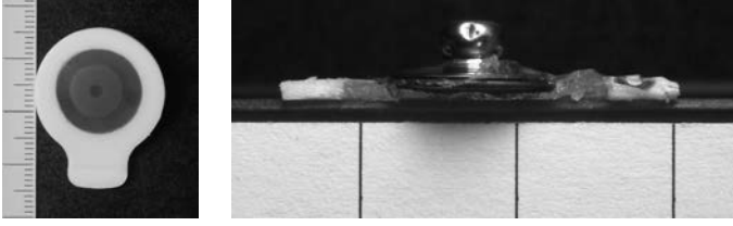
Fig. 5. Pictures of the ECG gel electrodes. On the left, view from the bottom; on the right, a lateral cross-section image, in which the gel area and the silver tip can be seen.
