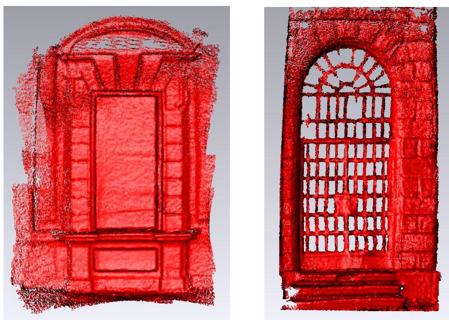
Figure 3. Screen-shots of the complete 3D ToF point cloud for both the surveyed windows.
