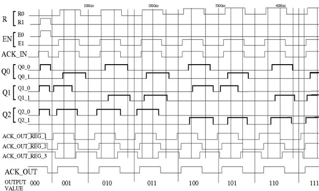
Fig. 12. NCL counter simulation results. Outputs are nodes  $Q0\_0$ ,  $Q0\_1$ ,  $Q1\_0$ ,  $Q1\_1$  and  $Q2\_0$ ,  $Q2\_1$ . They switch from the NULL (00) to the DATA (01 or 10) state. Output values are also reported in the bottom line in digital un-encoded format. The ACK\_OUT signal validates outputs.
