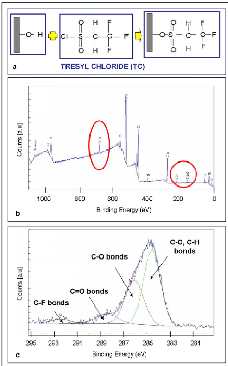
**Fig 2:** XPS survey spectrum (a) and detailed study of carbon region (b) for a thermo-chemically treated and functionalised sample
