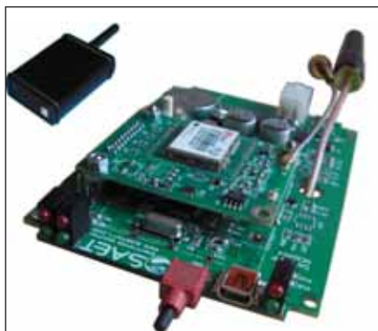
Fig. 2: A naked view of SAT-SURF (hardware)
