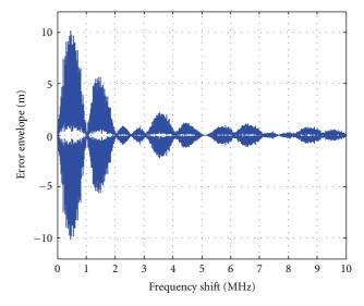
FIGURE 3: Interference Error Envelope in presence of a CW interference obtained for a coherent Early-Late discriminator with a correlator spacing of 0.4 chip with a BPSK signal.
