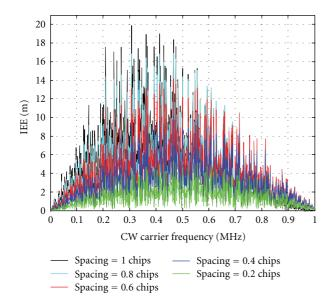
FIGURE 8: Comparison of IEE curves obtained varying the coherent Early-Late discriminator spacing (zoom on Figure 2).
