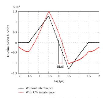
FIGURE 1: GPS L1 signal (BPSK) discrimination function distortion due to the presence of a CW interference (coherent Early-Late discriminator with 1 chip spacing, integration time equal to 4 ms).
