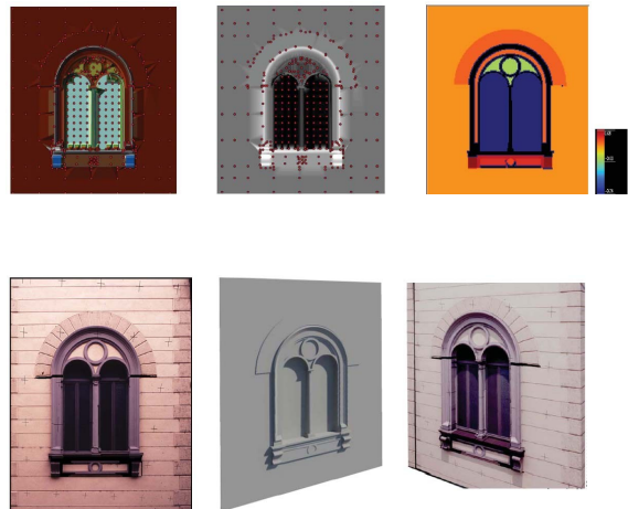
Figure 3: different level of details of documentation requirements demand different survey system. Continuous surfaces acquiring methods request suitable classification of elements strategies. In the picture sequence different processing phases (stereoplotting, dem processing, ortophoto and orthophoto 3D processing for a double lancet window). elaboration Presti.G.
