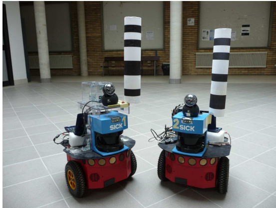
Figure 10: Robots P3-DX used for real tests. A bar code marker is used to distinguish the robots.
