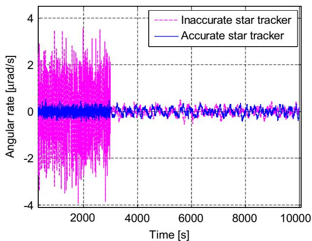
Fig. 13. Angular rate under different star tracker accuracies.
