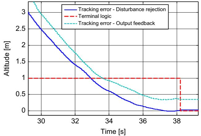
Fig. 7. Convergence of the 'true' terminal altitude error.
