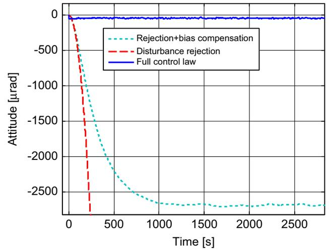
Fig. 10. Attitude drift for different control laws.
