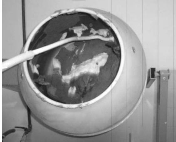
Fig. 2. Soil conditioning in the mixer bowl
