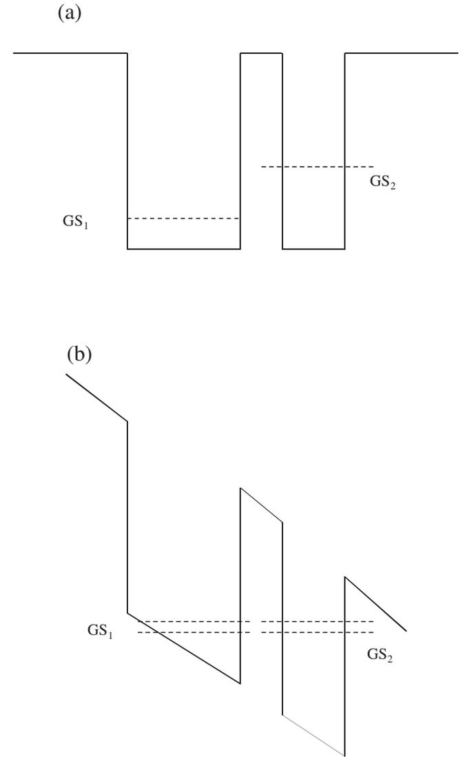
**Fig. 4.** (Color online) (a) Energy levels position in conduction band, for GS of two stacked QDs (or two adjacent QWs as well), with flat bands in absence of electric field (build-in potential is not considered here, for simplicity). (b) Electric field can be used to fine-tune the levels position. If spacers between QD layers (or barriers between QWs) are thin enough, levels are coupled and split.
