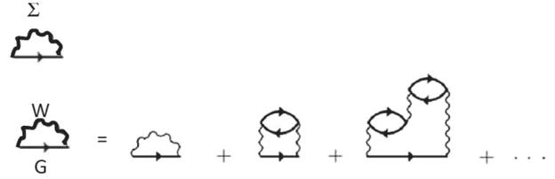
**Fig. 2.** The self-energy in a generally accepted approximation is represented by a propagator  $G$  multiplied by the interaction  $W$  and integrated over internal exchanged momentum. The effect of potential screening can be visualized as a summation over infinite ladder contributions.
