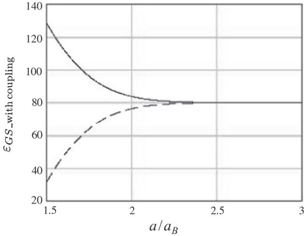
**Fig. 5.** (Color online) GS energy level splitting by effect of QD-QD coupling, for two stacked layers of self-assembled InAs/GaAs quantum dots, at null carrier density. Electron mass  $m$  has been set to 0.060 free electron mass. In abscissas,  $a/a_B$  is the layers separation in unit of Bohr radius  $\hbar/\sqrt{m\tilde{\epsilon}_{GS}}$  (here  $\approx 4$  nm).
