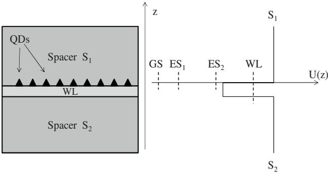
**Fig. 1.** On the left, a sketch of a WL-QD layer grown by Stranski-Krastanov method is shown. On the right, conduction band is shown with the confining potential  $U(z)$ , the WL bound level (substantially a very thin quantum well), ground state (GS) and excited states (ES) of quantum dot.
