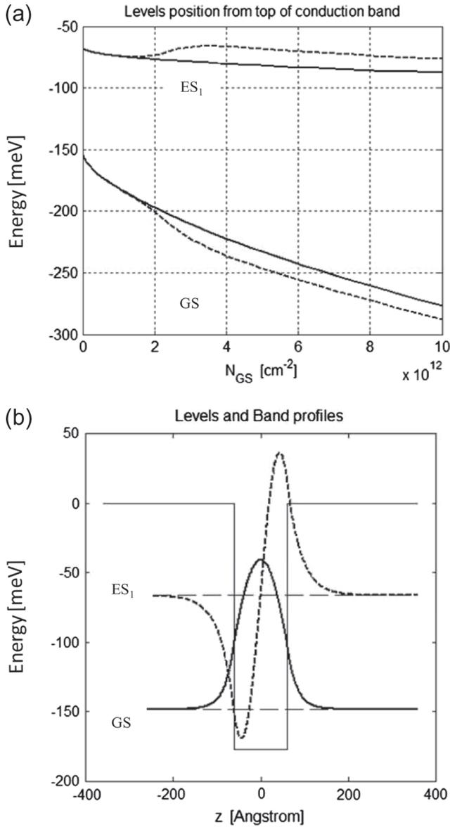
**Fig. 3.** (a) Energy levels position for GS and  $ES_1$ , with off-diagonal self-energy contribution (dashed lines) and disregarding them (solid), as a function of the GS two-dimensional carrier density. (b) Well/barrier potential profile, with unperturbed (0-density) levels position, GS (solid) and ES (dashed) eigenfunctions in the  $z$ -direction.
