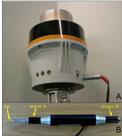
Figure 1 - A) iGPS transmitter. B) Two sensor vector bar
