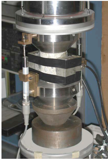
Figure 1: Apparatus adopted for compression tests (a); Stress and cumulated event number versus time (b).
