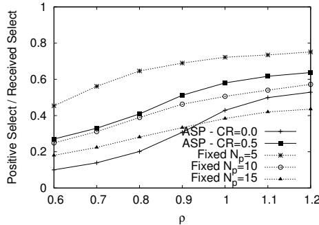
Figure 10. Fraction of positive select messages versus load.
