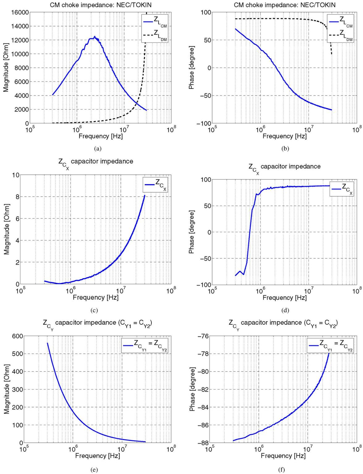
Fig. 8. Measured impedance of the chosen filter components. (a) and (b) CM choke (NEC/TOKIN). (c) and (d)  $C_X = 1.5\text{-}\mu\text{F}$  capacitance. (e) and (f)  $C_{Y1} = C_{Y2} = 1000\text{-pF}$  capacitances.
