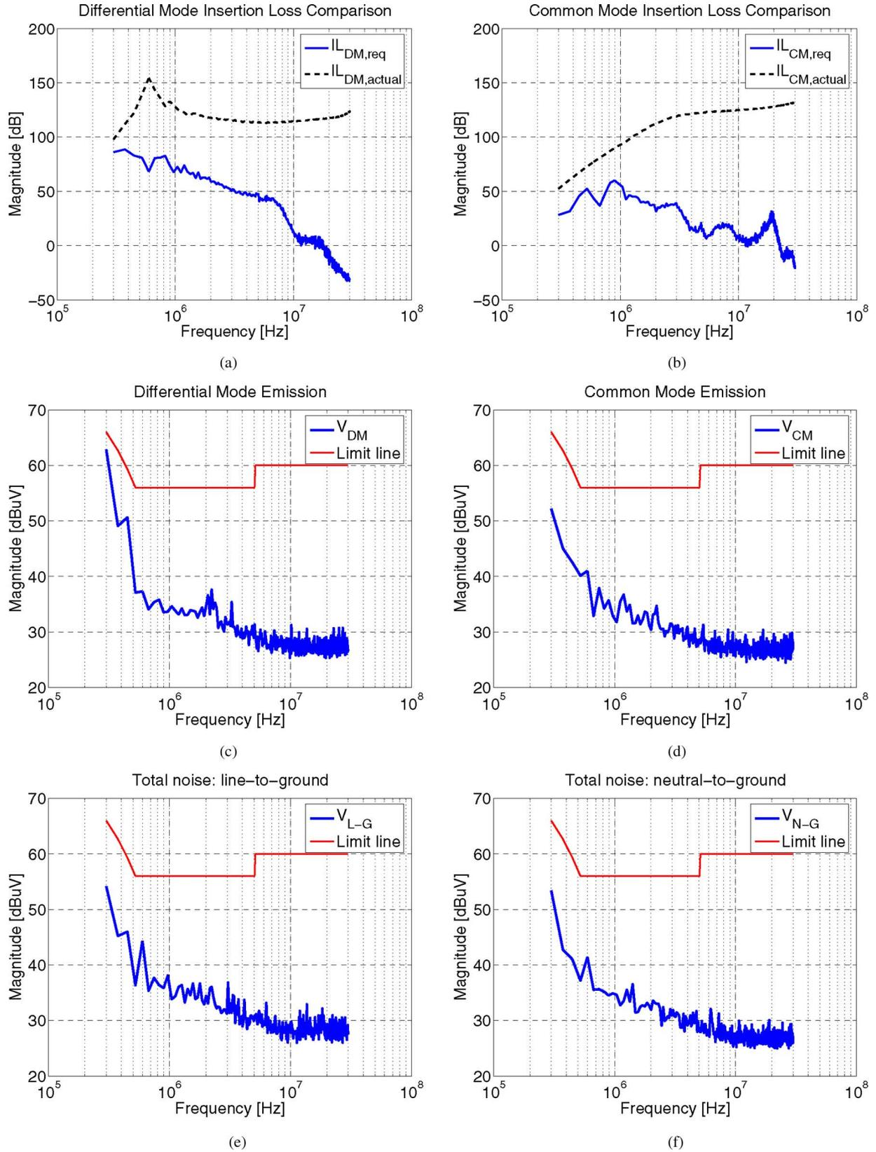
Fig. 9. Effect of the insertion of the EMI filter. (a) Required and designed DM insertion losses; (b) required and designed CM insertion losses; (c) measured DM conducted emissions with filter; (d) measured CM conducted emissions with filter; (e) measured total conducted emissions for line-to-ground; (f) measured total conducted emissions for neutral-to-ground.
