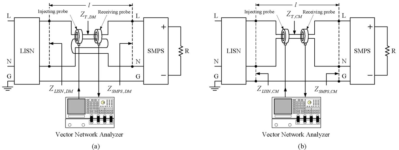
Fig. 2. In-circuit measurement setup. (a) DM. (b) CM.
