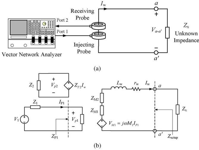
Fig. 1. (a) Conceptual two-probe in-circuit measurement setup. (b) Equivalent circuit of the measurement setup.
