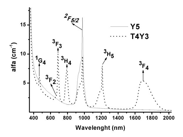
Fig. 4 - Absorption cross section of  $Yb^{3+}\,^2F_{5/2}$  in Y5 glass (group I).
