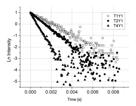
Fig. 11 – Fitting and experimental values of Yb lifetime from group I glasses using equation (1).
