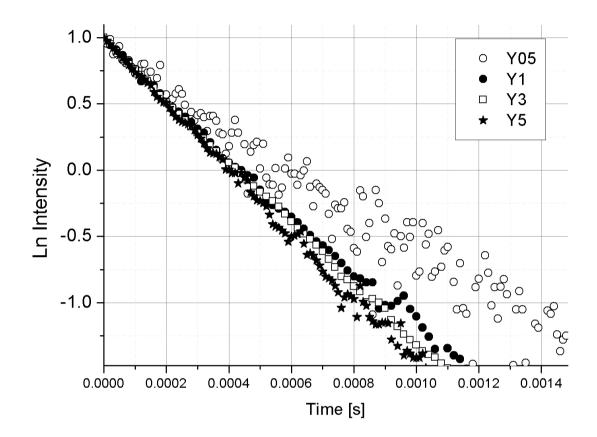
Fig. 10 - Tm  ${}^3F_4$  lifetime for group II glasses by pumping at 785 nm.
